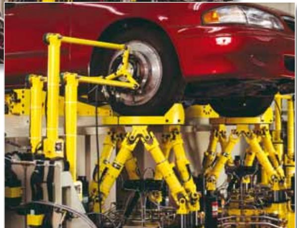
The system performs suspension dynamic tests by moving the tire platforms at frequencies up to 35 Hz with various combinations of load and stroke control. For dynamic tests the vehicle body can be clamped, free, or restrained with an optional cg restraint system. The latter allows you to evaluate suspension performance under simulated road and body force conditions.
