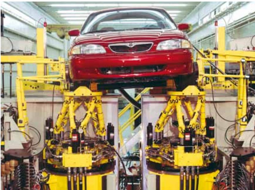
MTS Dynamic K&C System measure both static and dynamic kinematic and compliance deflection properties of vehicle suspension
